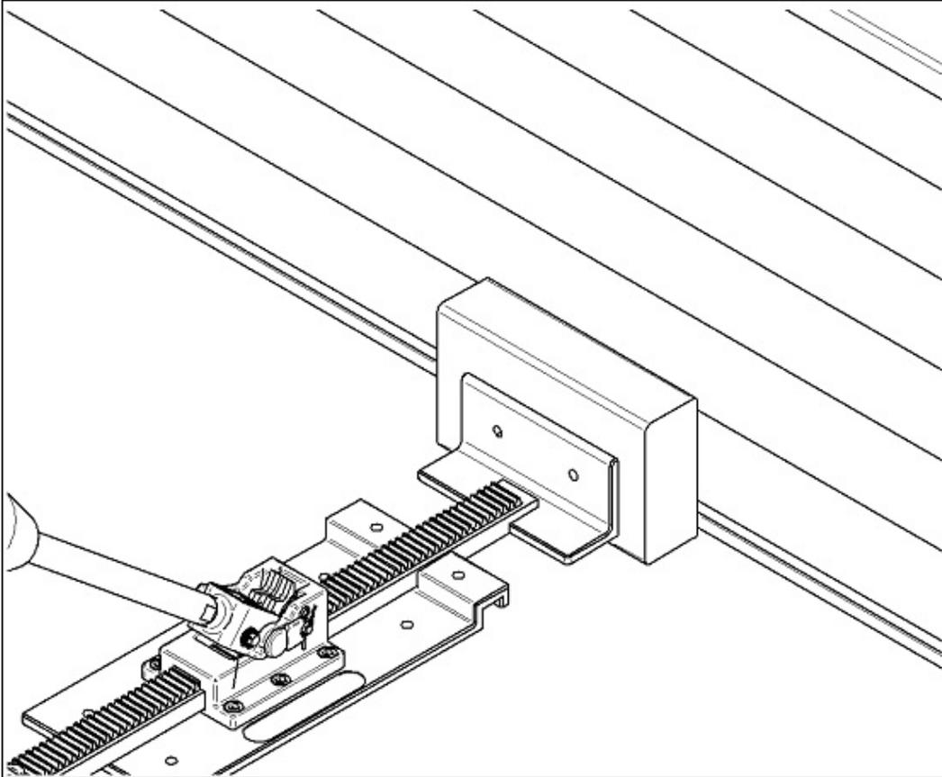
The Prim-Jack will work on any thickness of flooring without damaging the flooring surface. The non-marring base is designed to protect the flooring surface by keeping the metal components of the Prim-Jack from coming into contact with the floor. The Prim-Jack can be used next to the wall at stud locations or anywhere on the floor using the appropriate tool positioning and configuration.
