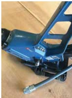
**2** Your air hose should have a minimum of 150 psi (10.6 kg/cm<sup>2</sup>) working pressure rating and be fitted with a quick-disconnect fitting at the tool.
