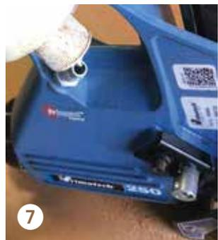
**7** Lubrication requirements are specific to your specific nailer and working conditions. Lubrication requirements from manufacturers may vary from two to four drops of oil every eight hours of use to two to four drops per week.
